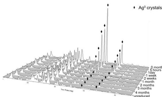
Fig. 3. XRD patterns of NO<sub>2</sub> aged Ag<sup>0</sup>Z for different periods and AgZ.
