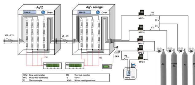
Fig. 1. The continuous-flow aging system.
