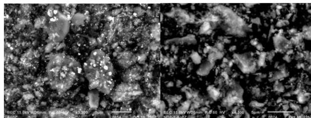
Fig. 4. SEM (backscatter electron) image for Ag<sup>0</sup>Z (left) and Ag<sup>0</sup>Z aged in NO<sub>2</sub> for 2 months (right). The bright dots observed on the Ag<sup>0</sup>Z image are Ag<sup>0</sup> particles which are not found on the NO<sub>2</sub> aged Ag<sup>0</sup>Z.
