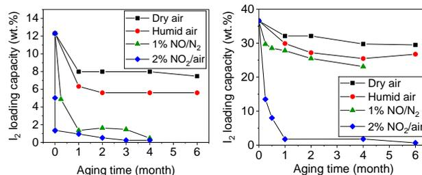
Fig. 5. Iodine adsorption capacity of Ag<sup>0</sup>Z (left) and Ag<sup>0</sup>-aerogel (right) as a function of aging time.
