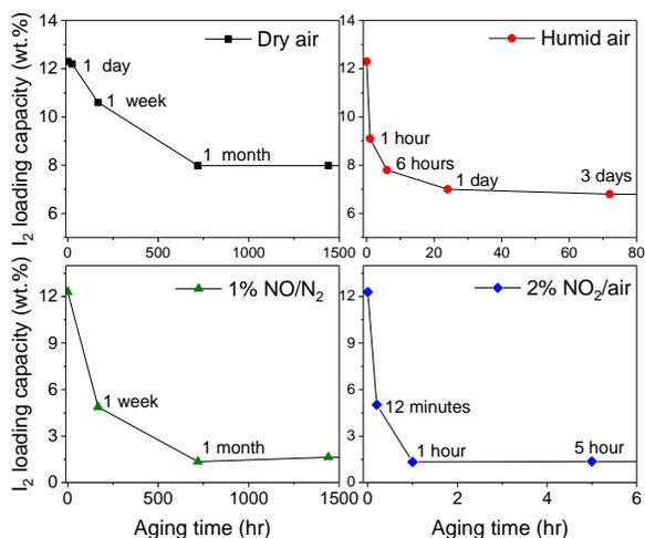
Fig. 6. Kinetic data of Ag<sup>0</sup>Z aging in dry air, humid air (dew point of -15°C), 1% NO/N<sub>2</sub> and 2% NO<sub>2</sub>/air at 150 °C.
