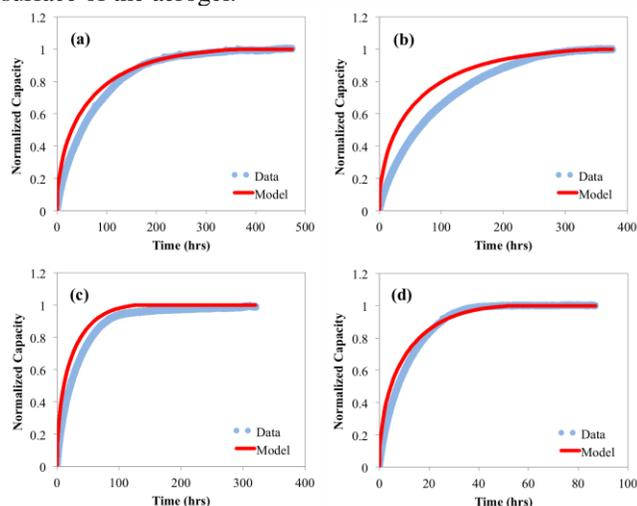
Fig. 2. Iodine uptake rate predictions in Ag<sup>0</sup>Z pellets at various temperatures (T) and iodine concentrations (C), without aging effects. (a) T = 100 °C and C = 1.3x10<sup>-3</sup> kPa, (b) T = 150 °C and C = 1.4x10<sup>-3</sup> kPa, (c) T = 150 °C and C = 3.7x10<sup>-3</sup> kPa, and (d) T = 200 °C and C = 8.8x10<sup>-3</sup> kPa.
