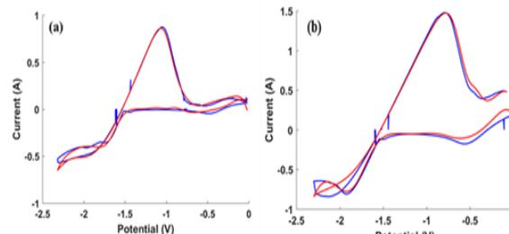
Fig. 7. Comparison of CV plot for (a): 7.5 wt%  $UCl_3$  at 450 mV/s, (b): 10 wt% at 1700 mV/s.
