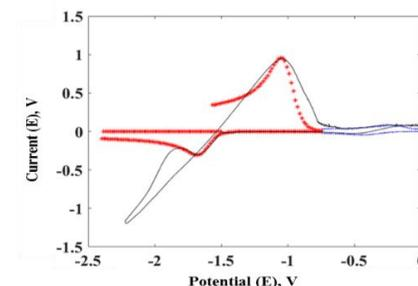
Fig. 3. CV of 10 wt%  $\text{UCl}_3$  in LiCl-KCl eutectic at 773K with 200 mV/s.
