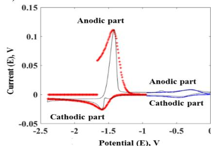
Fig. 2. Cyclic voltammetry of 1 wt%  $\text{UCl}_3$  in LiCl-KCl eutectic at 773K with 100 mV/s.
