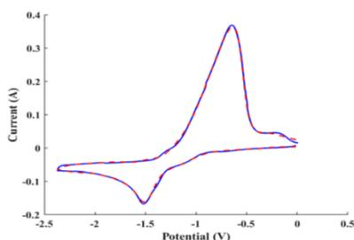
Fig. 6. Comparison of CV plot for 0.5 wt%  $ZrCl_4$  in LiCl-KCl eutectic at 773K with 450 mV/s with [9, 15, 10]-18 implementation.
