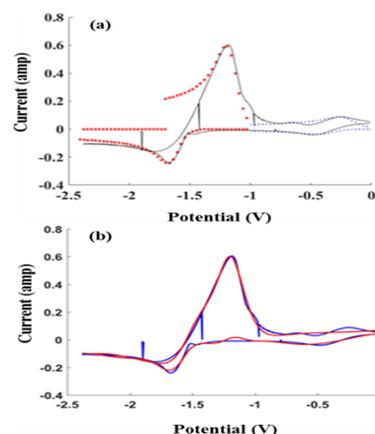
Fig. 8. Cyclic voltammery of 5wt%  $UCl_3$  in LiCl-KCl eutectic at 773 K with 400 mV/s, (a): diffusion mode, (b): ANI method.
