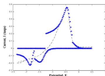
Fig. 5. Cyclic voltammery of 1 wt%  $ZrCl_4$  in LiCl-KCl eutectic at 773K with 300 mV/s.
