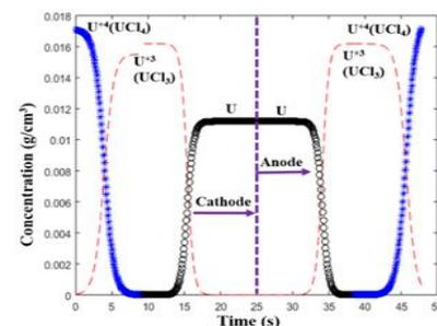
Fig. 4. Reduced and oxidized species for 1 wt%  $\text{UCl}_3$  in LiCl-KCl eutectic at 773K with 100 mV/s.
