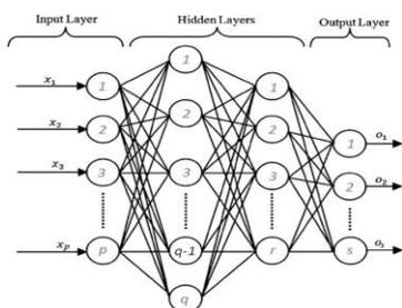
Fig. 1. Multi-layer perceptron schematic [14].
