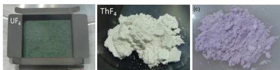
Fig. 1. Photos of the final products UF<sub>4</sub>, ThF<sub>4</sub> and PuF<sub>3</sub> (from left to right)
