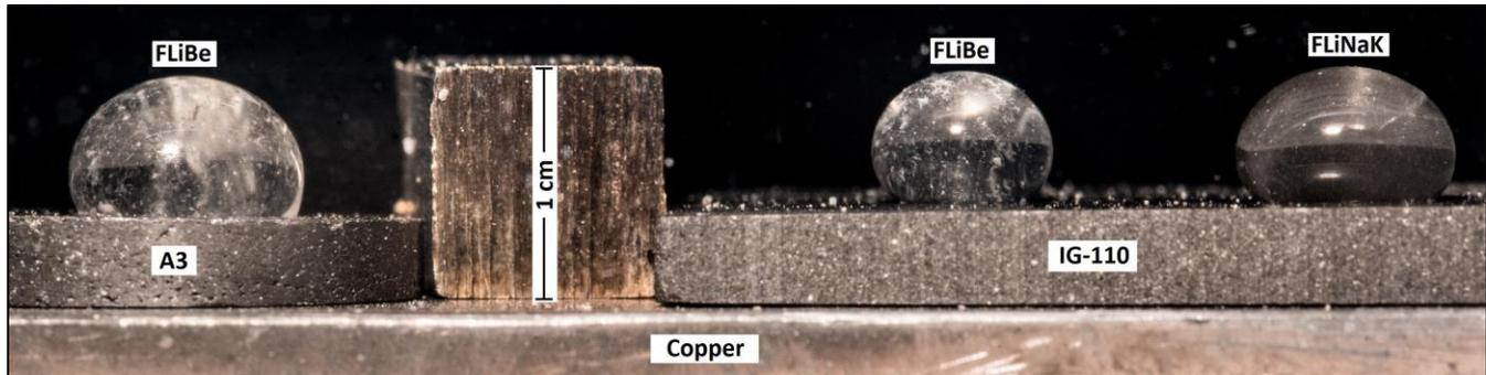
Figure 5: FLiBe and FLiNaK sessile droplets at 500°C on matrix graphite A3 and nuclear graphite IG-110 at UW-Madison.
