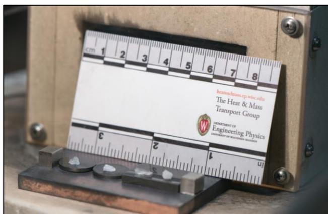
Figure 3: Solid FLiBe and FLiNaK samples on nuclear graphite, on a copper block, above a furnace. The insulating calcium-silicate lid is displayed behind the samples.
