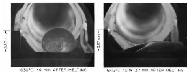
Figure 2: FLiBe is non-wetting on graphite in dry helium (left) but wets graphite at 10 ppm  $\text{H}_2\text{O}$  in helium (right)[3].
