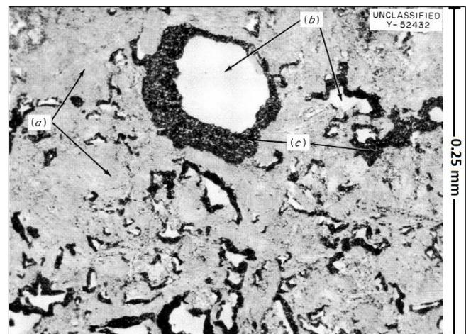
Figure 7: Microstructural details of CGB from MSRE. (a) graphitized coke particles. (b) and (c) structures developed through impregnations and heat treatments [12].
