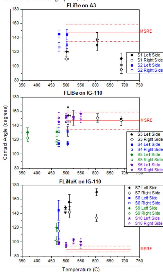
Figure 4: FLiBe and FLiNaK contact angle on graphite.
