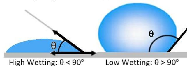
Figure 1: Contact angle measurements from sessile drops.
