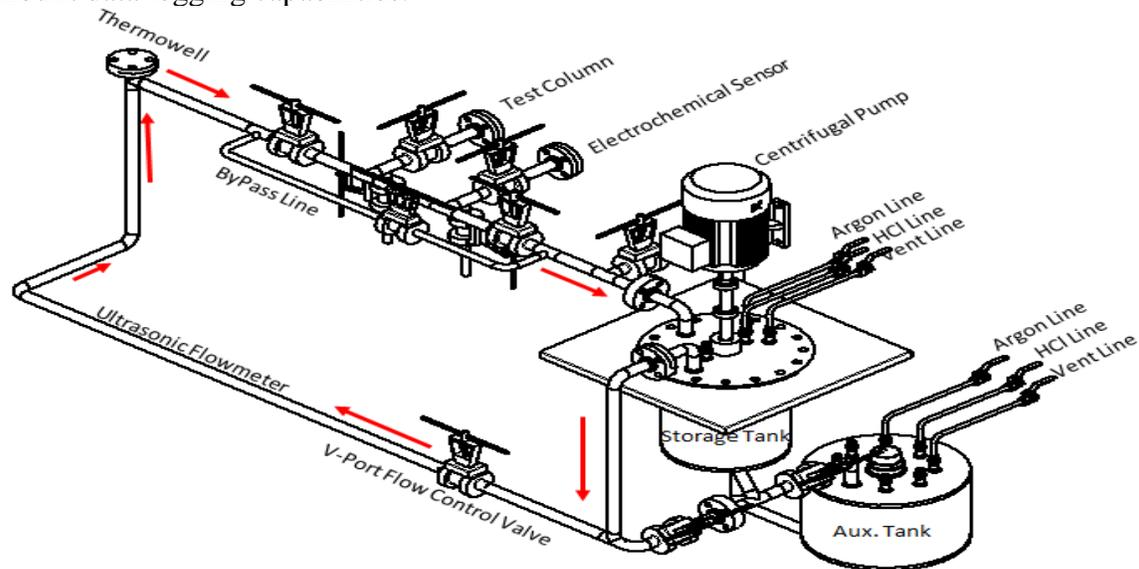
Fig. 1: A 3D layout of molten salt loop.
