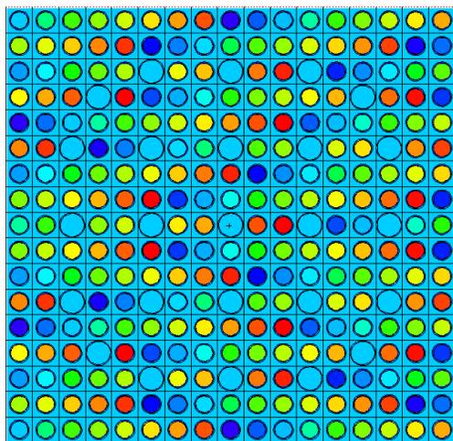
Fig. 1. MCNP Graphic of 17x17 PWR Fuel Assembly.
