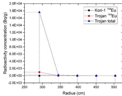
Fig. 4. Kori unit 1 bioshield average <sup>154</sup>Eu activity comparing with Trojan [3] nuclear power plant
