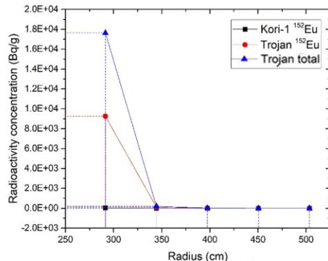
Fig. 3. Kori unit 1 bioshield average <sup>152</sup>Eu activity comparing with Trojan [3] nuclear power plant
