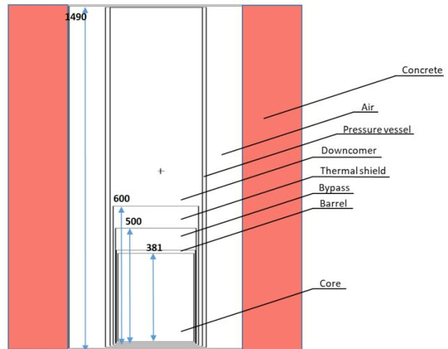
Fig. 1. Kori-unit 1 reactor vessel geometry [1] (cm)
