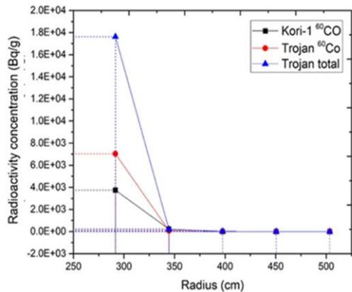
Fig. 5. Kori unit 1 bioshield average <sup>60</sup>Co activity comparing with Trojan [3] nuclear power plant
