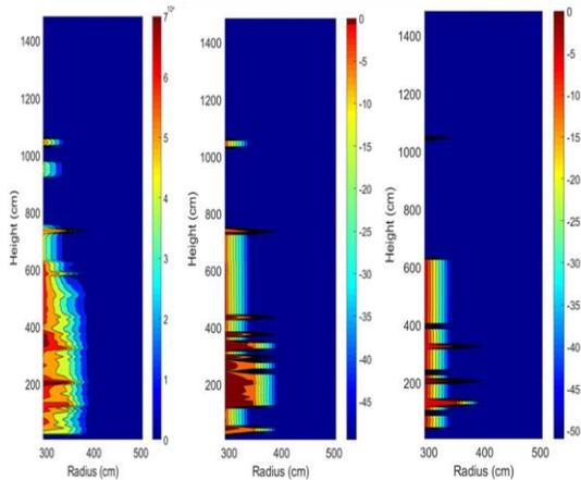
Fig. 2. Kori unit 1 bioshield radioactivity concentration <sup>60</sup>Co Bq/g (Left) <sup>152</sup>Eu Bq/g (Middle), <sup>154</sup>Eu Bq/g (Right)
