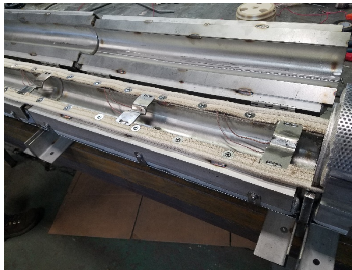
Fig. 3. Two zones of the tube shell with the lid open and the rod supports visible.
