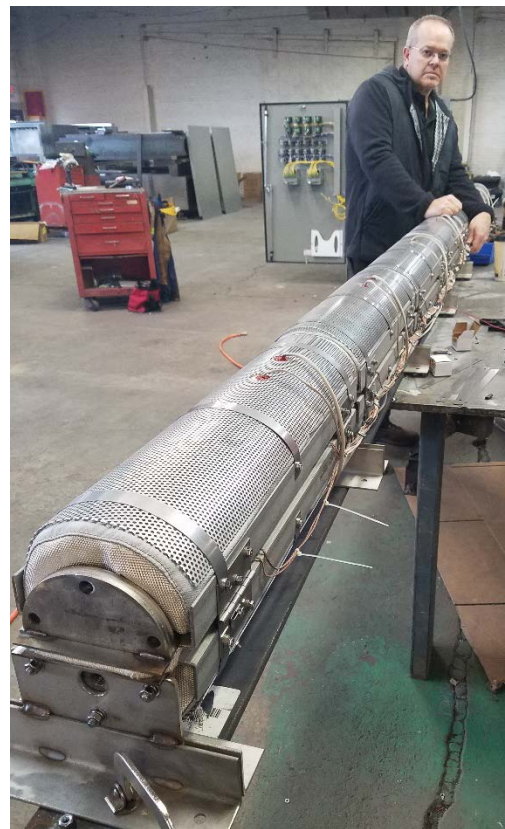
Fig. 1. The SFRHTO tube shell with its seven modular zones. The power and thermocouple cables for the heating blankets are visible at the top center of each zone.
