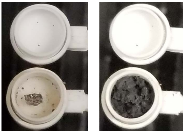
Fig. 3. On the left is pure uranium prior to analysis in the TGA. On the right is pure uranium after analysis.
