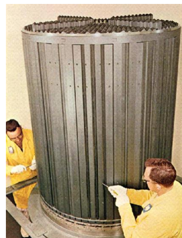
Figure 3: Graphite core of the MSRE.
