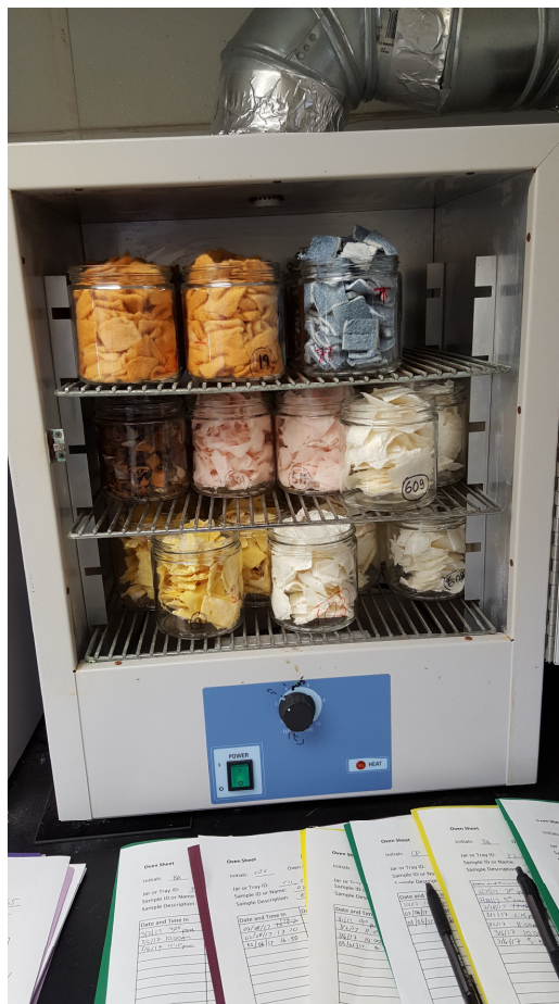
Fig. 2. Several samples of different organic wipes mixed with different concentrations of \text{KNO}_2 solutions awaiting for testing in oven.
