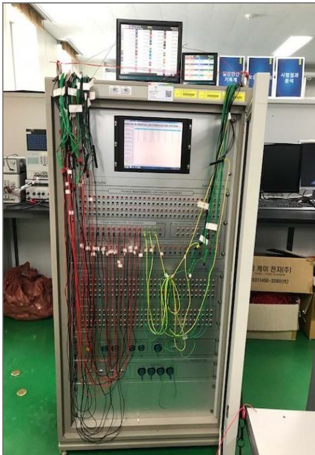
Fig. 5. Simultaneous testing of KR-2000 recorder and KR-3000 recorder
