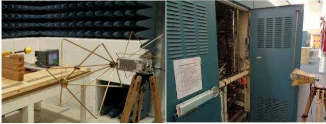
Figure 1. Laboratory Radiated Susceptibility Testing of the Digital Recorder (left) and In-situ Radiated Emissions Site Survey in the Control Room (right).
