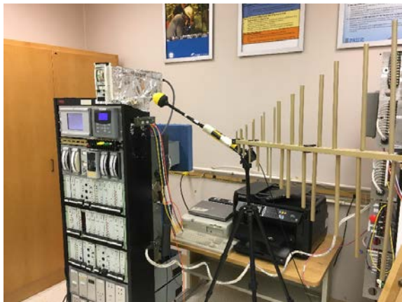
Figure 4. Test Setup for Immunity Testing in a Laboratory at Nine Mile Point
