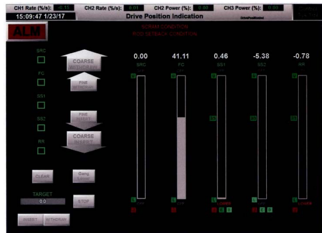
Figure 2. The Main Operator Screen, which was designed to look much like the original operator control panel. [1]
