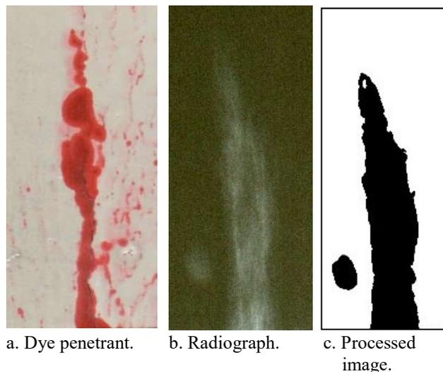
Fig. 1. Crack 6a shown by different techniques
