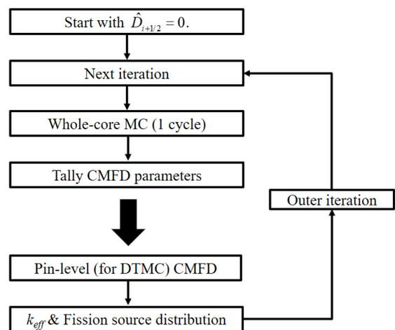
Fig. 1. CMFD accelerated MC neutron transport flow chart
