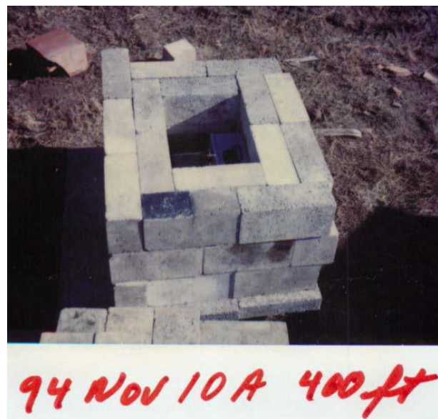
Fig. 3. Concrete Block Shield for CAAS Testing.
