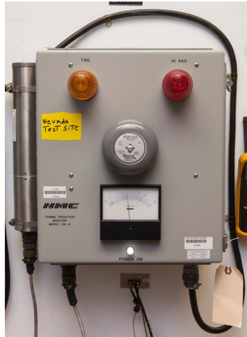
Fig. 1. Nuclear Materials Corporation GA-6 Radiation Detector.
