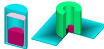
Fig. 5. Can-bag-can (left) and glovebox radiation shield (right) branch case models.
