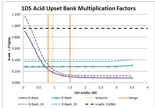
Fig 3. Neutron Multiplication of D and E Banks During Upset Conditions.
