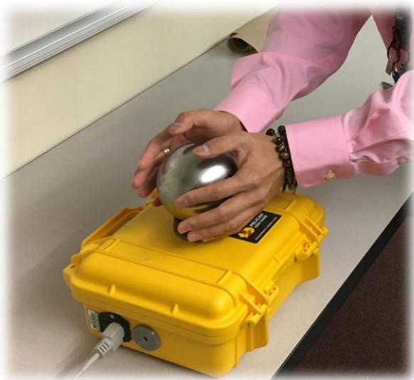
Fig. 1. Demonstration of increased reactivity due to reflection using the reactivity simulator.
