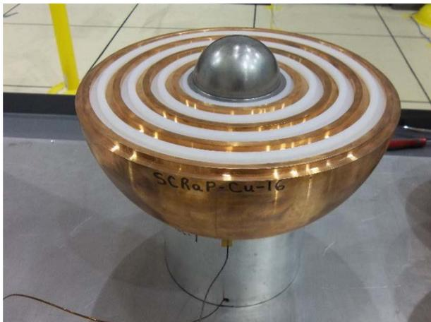
Figure 2. Configuration 7, which shows the various layers of polyethylene and copper, as well as where the thermocouples enter the system.
