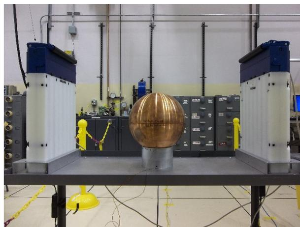
Figure 1. Overview of Configuration 7, including the multiplicity detectors.
