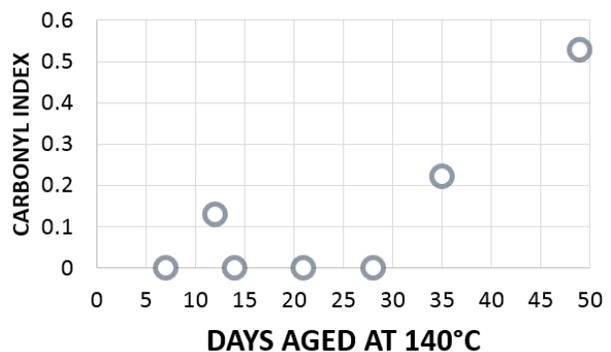
Fig. 6. CI versus days at 140°C for CPE jacket material. Indenter modulus of the cable segment CPE jacket, plotted in Fig. 7, is more sensitive to the thermal aging, tracking aging after less than 15 days at 140°C.
