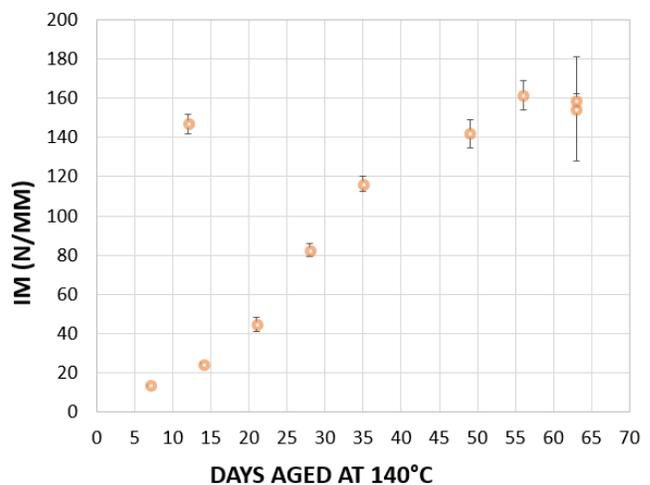
Fig. 7. Indenter modulus (IM) versus days at 140°C for CPE jacket material on cable segments.
