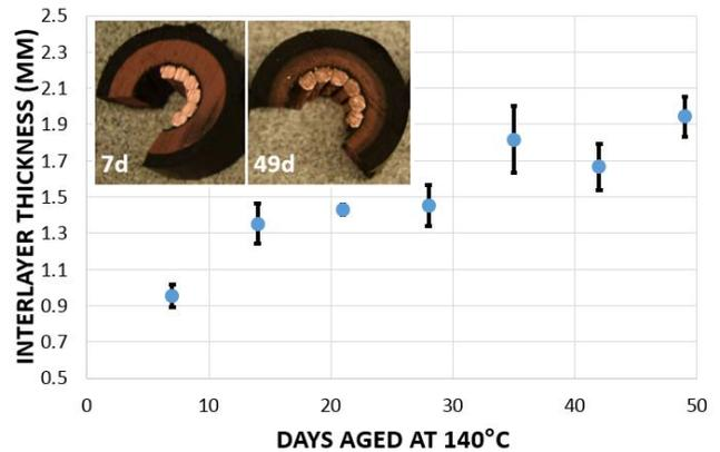
Fig. 5. Interlayer thickness of cable segments aged at 140°C.
