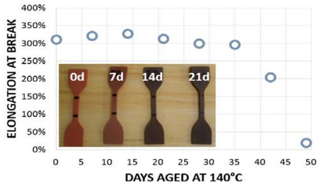
Fig. 1. EAB versus days at 140°C for EPR mat specimens.
