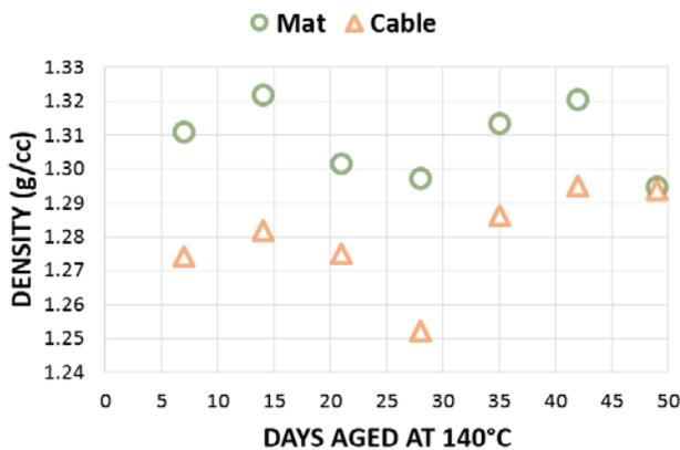
Fig. 4. Density versus days at 140°C for EPR samples.
