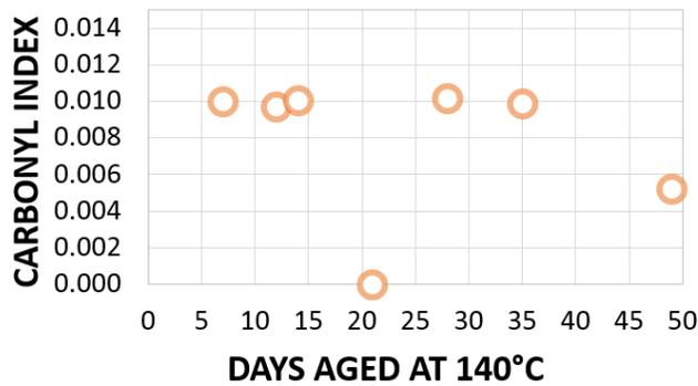
Fig. 3. CI versus days at 140°C for EPR cable material.
