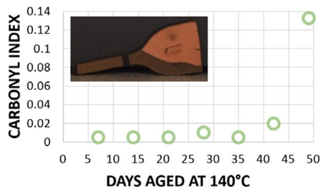
Fig. 2. CI versus days at 140°C for EPR specimen interiors.
