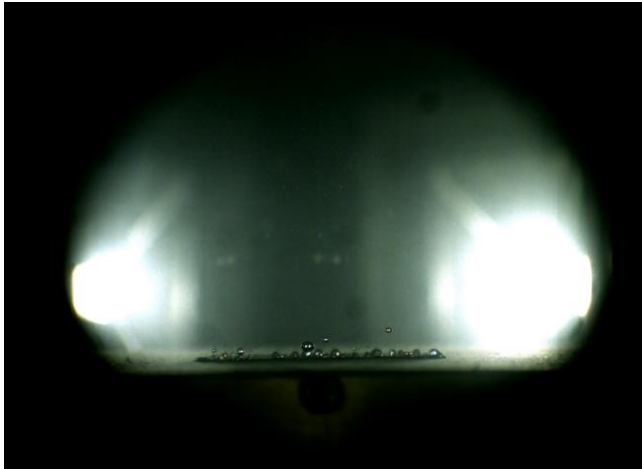
Fig. 5 Onset nucleate boiling ( \Delta T_{sat} = 21.47K , q'' = 1.7 \times 10^4 W / m^2 )
