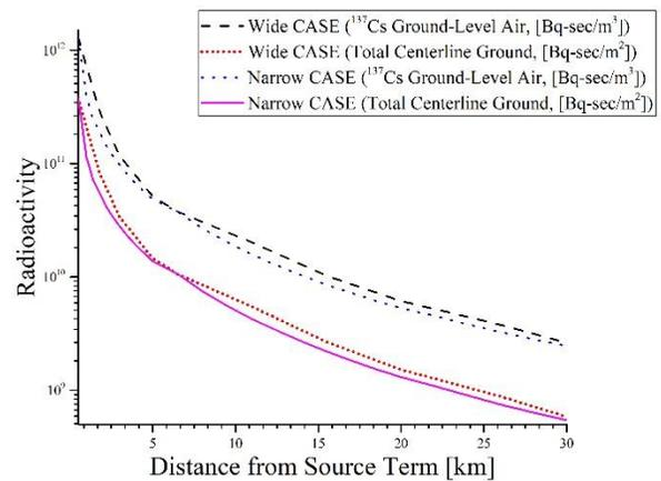
Fig. 3. Radioactivity according to the Distance from the Source Term.
