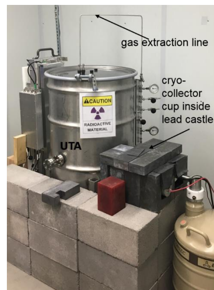
Fig. 1. Picture of prototype Gas Extraction Module (GEM) attached to UTA, comprised of an extraction line, series of valves and gauges, and a cryogenic collection cup (inside the lead castle).
