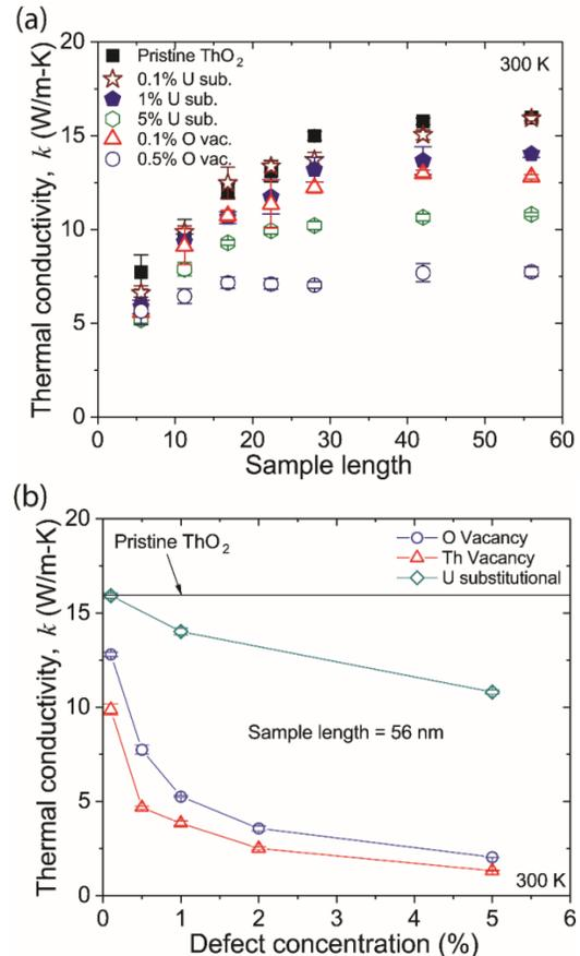
Fig. 3. Thermal conductivity of ThO<sub>2</sub> with O vacancy, Th vacancy, and U substitutional.
