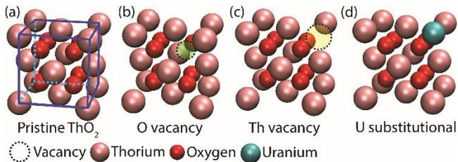
Fig. 2. Various defects in ThO<sub>2</sub> simulated in this study.
