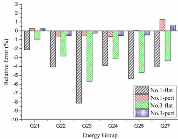
Fig. 1. Relative cross section errors in region No.1 and No.3 by two approaches (flat: flat source assumption. pert: temperature perturbation technique.).
