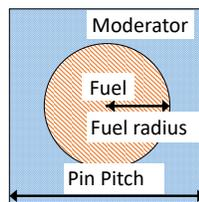
Fig. 1. Example of calculation geometry (reflective boundary condition).
