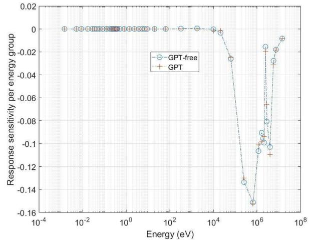
Fig. 1. Comparison of group-wise sensitivity coefficients of a generalized response with GPT and GPT-free.
